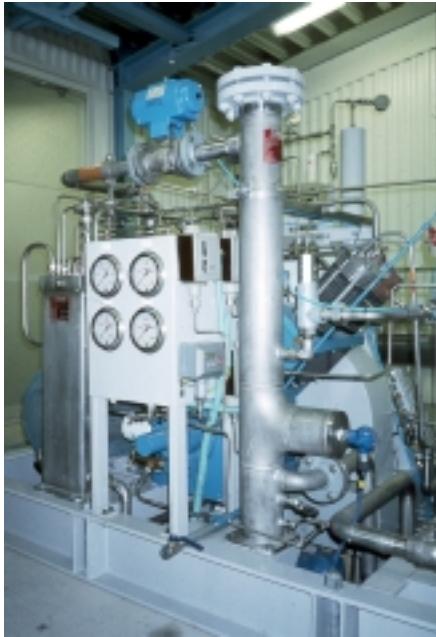
A compact unit that scrubs and compresses biogas for use as an alternative motor fuel
