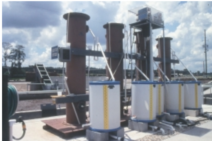
Pilot-scale anaerobic filter at the University of Florida (photo credit: Ann C. Wilkie)
